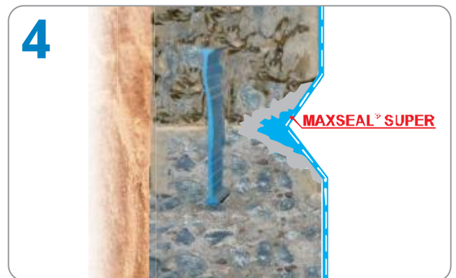
4 WATERPROOFING APPLICATION MAXSEAL ® SUPER THI CÔNG CHỐNG THẤM MAXSEAL ® SUPER
